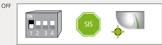
RELAY 2: REOPENING-impuls on the closing side of the door
